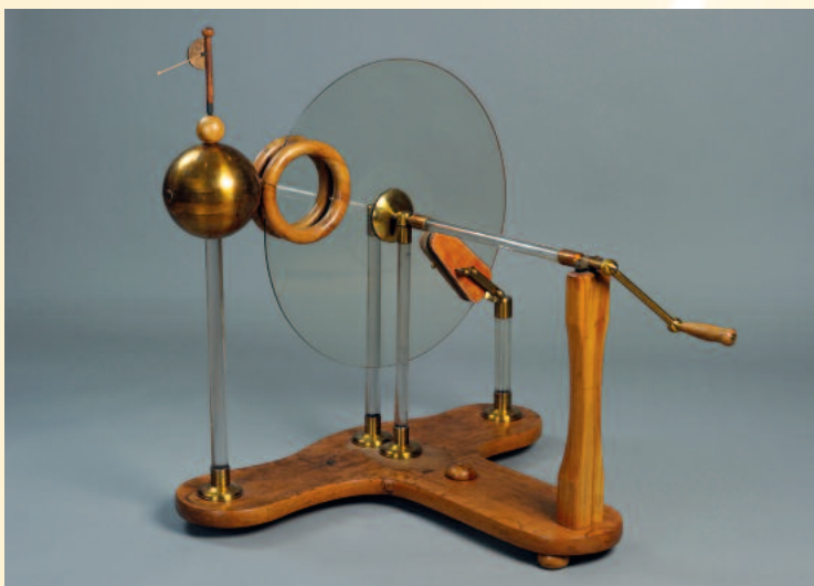
Frictional electrical machine with a rotating glass plate from Lichtenberg’s laboratory. The separated charge is rotated and picked up by a needles at the spherical capacitor. The charged status is indicated by the vertical position of the straw pointer. Photos: Manfred Mahn (right), Frank Stefan Kimmel (left)
